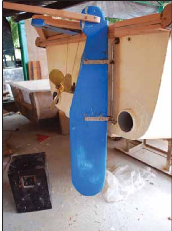
Figure 121 Detail of the emergency rudder to be used with sail.
