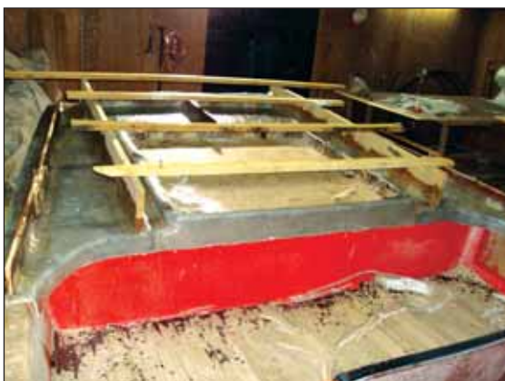
Figure 119 Final stage of the making of the mould for the aft deck.
