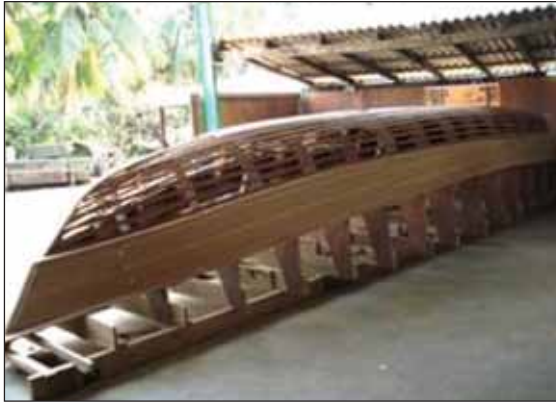
Figure 46 Applying veneer ply skin.
