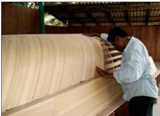
Figure 48 Diagonal strips for a curved surface.
