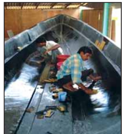
Figure 66 Rubbing down with water emery.
