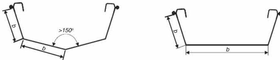
SMALL BOATS WITH HARD CHINES. TRANSVERSE FRAMES WITH GREATER SPACING THAN b
