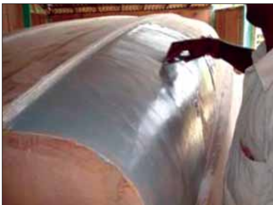
Figure 51 Applying autograde putty.
