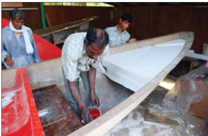
Figure 122 The fore and aft decks are assembled the same way by seating the decks on the hull flange after placing the required polystyrene buoyancy blocks under the deck.
