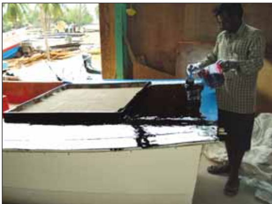
Figure 118 The first layer of gelcoat being applied on the deck plug.
