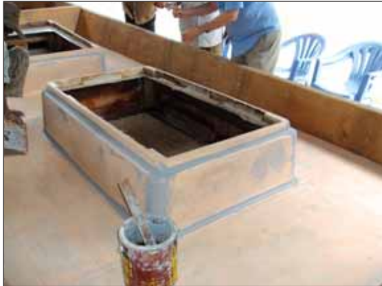
Figure 105 Application of modelling clay.
