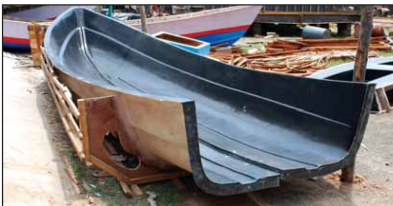
Figure 67 The completed split mould (without the transom).
