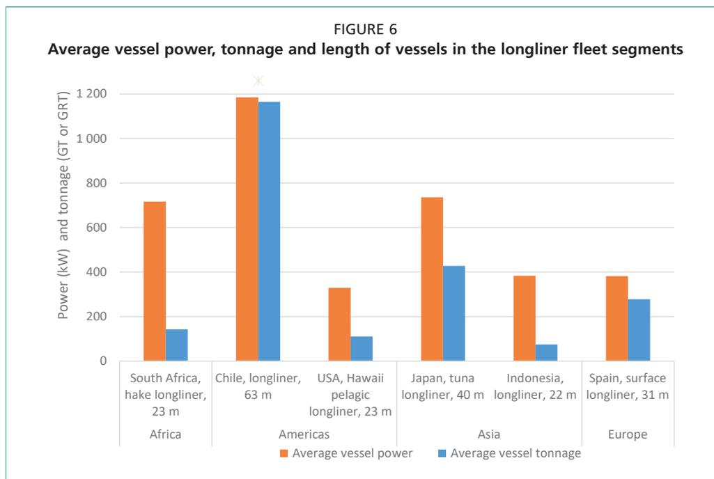
The six longliner fleet segments for which tonnage and engine power information was available showed significant variation in terms of average vessel size. The average vessel length ranged from 22 m to 63 m. Engine power ranged from 329 kW for average vessels in the Indonesian longliner fleet segment to 1 185 kW for the average Chilean longline vessels, while tonnage ranged from 75 tons to 1 165 tons. The largest longliner vessels among the fleets surveyed were found in Chile.
