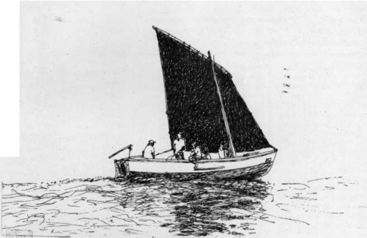
Above: IND-20 sailing with Dipping Lug rig. Below: Kattumaram being carried ashore.
