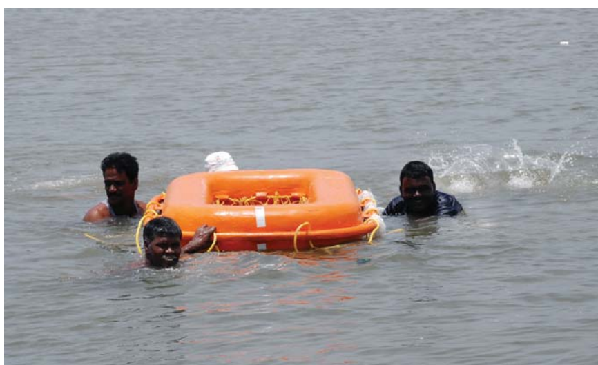
FRP life float for larger boats as an alternative to an inflatable life raft*
