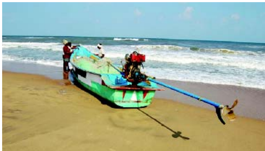
A traditional Andhra boat with an outboard motor fitted with long-tail propulsion unit
