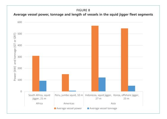
The review covered four squid jigger fleet segments. Indonesia and the Republic of Korea's squid jigger vessels were the largest, particularly with regard to engine power.
