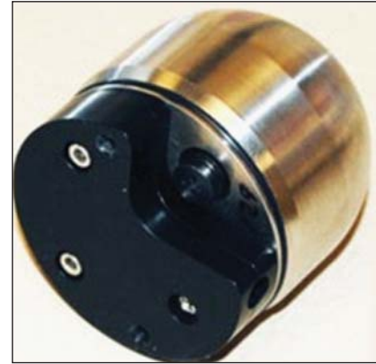
Figure 5. SBE 63 optical dissolved oxygen sensor
