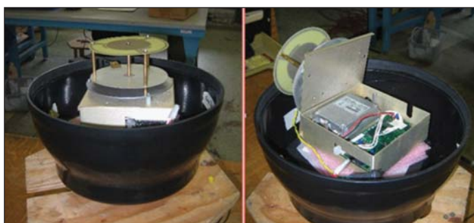
Argos-3 Kenwood PMT integrated in a SVP drifter
