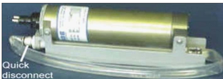
Figure 1. SBE 4 Conductivity sensor with Tygon® loop used for storing the sensor
