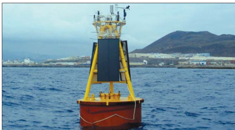
ESTOC moored buoy using Argos-3 interactive mode in Canaries
