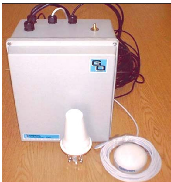
Figure 3: Satellite deck box w/ GPS & Iridium Antenna
