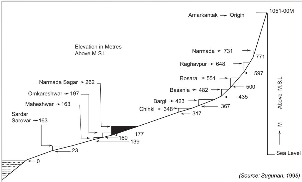
**Fig.3: Cascade of reservoirs on the river Narmada**
